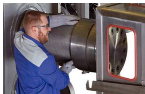
Screen assembly (CSC-R installed for horizontal melt flow)
